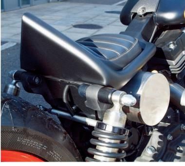
Rocket Bobs: minimal sag and short but well damped travel using decent springs. It's born of Pete's involvement in building race bikes in a former life, and he's a firm believer that about an inch of wellcontrolled wheel movement is not only good for handling, but also can be more comfortable than a soft four inches - especially in concert with a decent seat using a clever composite foam structure.
