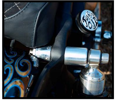
Alcantara faux suede. It sits above a horseshoe oil tank that Pete is less than happy with, but until he's worked out what to replace it with, he has fitted tunnels from the battery tray to the motor to take the leads from a Crane single fire coil, which shares that space with a Rocket Pack: Rocket Bobs' new Lithium Ion battery.
