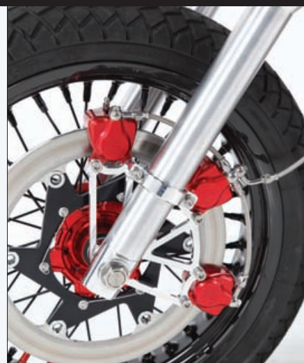
Detailing on Gas'd Rat extends to the bike's name being machined into the Harrison Billet supplied brake callipers
