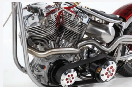
Details on the drivetrain include a sealed mercury cylinder inside the front engine pulley to dynamically balance the motor
