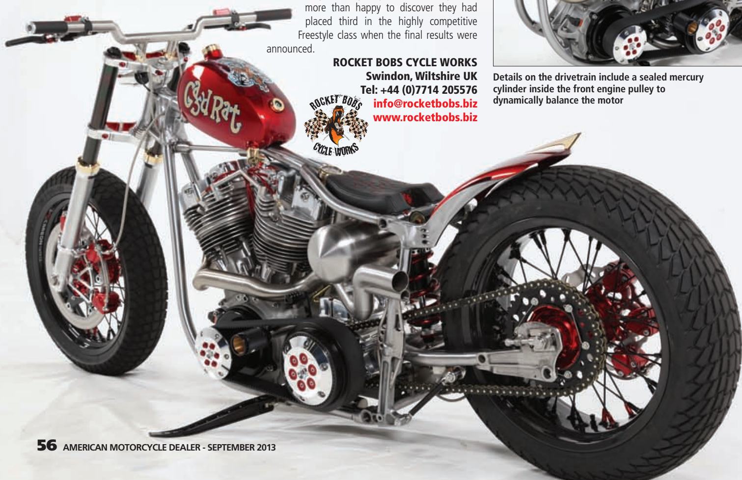
Each frame joint was taken apart and refinished before being TIG welded, while the addition of a stainless steel brace has been added to the headstock, too
