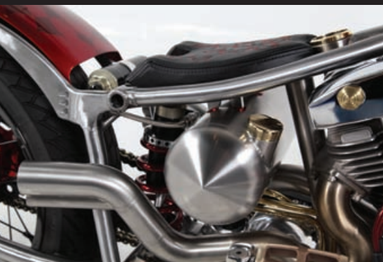
Hidden brackets were made to support the one-off stainless steel oil tank
